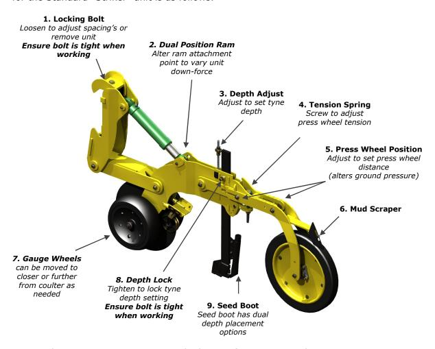
Due to having so many points and planes of variation each increment of movement with its primary and secondary effects is not listed here. Both the Simplicity "X-Bar" and "Striker" units have been built to have maximum versatility and each movement and variation can have different effects depending on planting conditions and soil type
