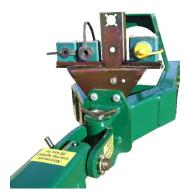
TR Air Seeder Hitched with Optional Rigid A-Frame Pull
